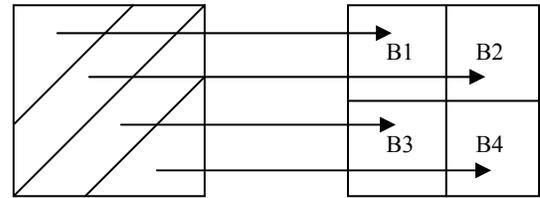
Figure 1. Mapping of DCT coefficients into 4 blocks
